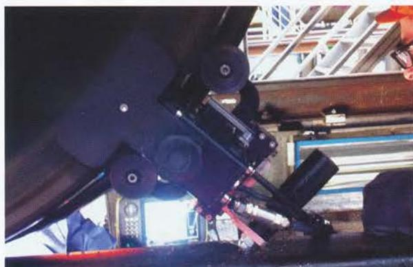
*Phased array ultrasonics for running gear inspections during railway maintenance operations*
