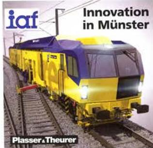
**Plasser & Theurer** will unveil its latest Unimat 09-4x4/4S E<sup>3</sup> universal tamping machine at the IAF track technology exhibition in Münster on May 30 – June 1. Fitted with an electric drive for the tamping vibration unit, this hybrid machine will be able to operate in fully electric or diesel-electric modes; it is also fitted with a Puritech filter system to permit diesel operation in tunnels.
